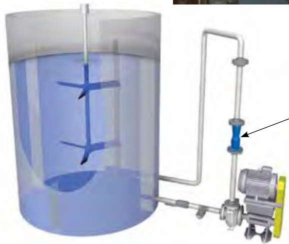
▲ Optimum installation with Leach Feed to the inlet of the injector and slurry returned into the base of the tank
