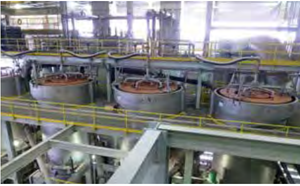
EFD Flotation columns in a mineral flotation application.
