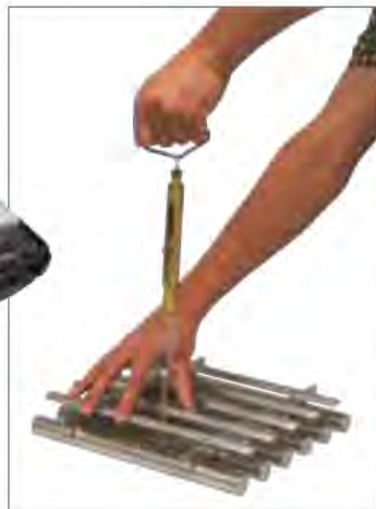
Pull Test Kits provide an accurate record of magnetic strength over time.
